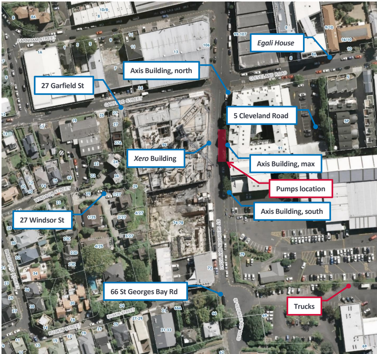
Figure 2: Emergency pump location and measurement locations
